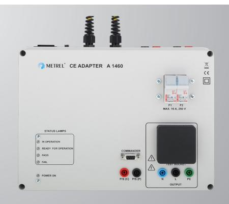
The A 1460 CE Adapter is an active switch or adapter intended to run AutoSequences® on electrical equipment in combination with the master instruments. The operation of CE test adapter is completely controlled by the master instrument, no user intervention during the tests is needed. I/O connections and LEDs for controlling the AutoSequence® flow are integrated. The adapter is protected against applying too high voltage to its outputs (HW and SW protection).
